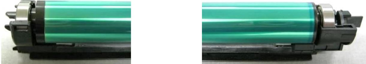
**16** Cover the new OPC drum with the black wrap removed during step 15 (protect it from light exposure).
