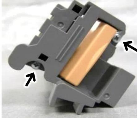
**18** Reattach and secure the rear bearing cover and the rear cover removed during step 2 and step 3.
