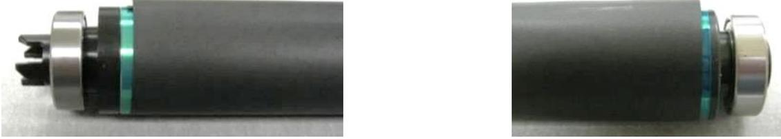
**15** Remove the black wrap from the new OPC drum and install it into the drum unit frame.
