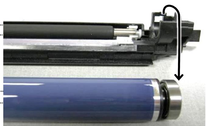
**8** Remove the 2 bearings from the used OPC drum and set aside.
