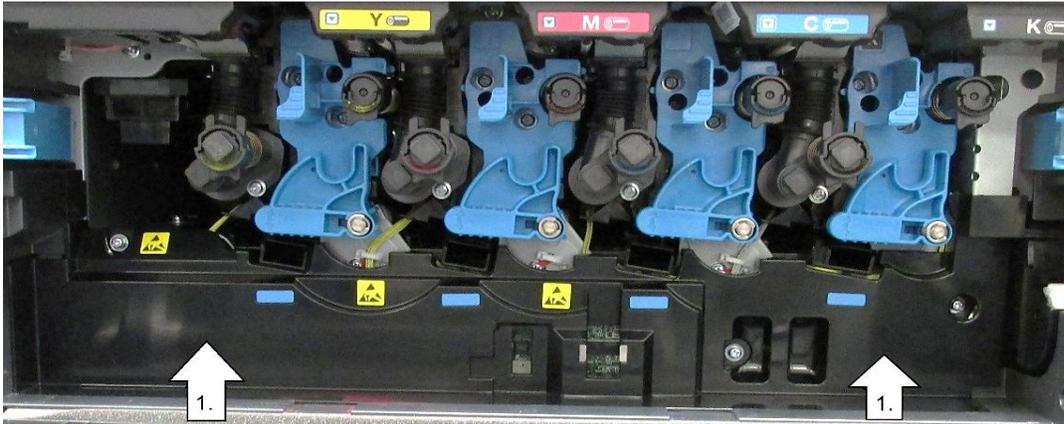
2. en Disconnect the desired developing unit connector from the FRB board.
