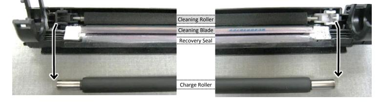
10 If replacing the drum cleaning blade, remove the 2 screws securing the plastic charge roller housing to the drum unit frame and remove the charge roller housing. Set the housing and 2 screws aside. If not, go to Step 13.
