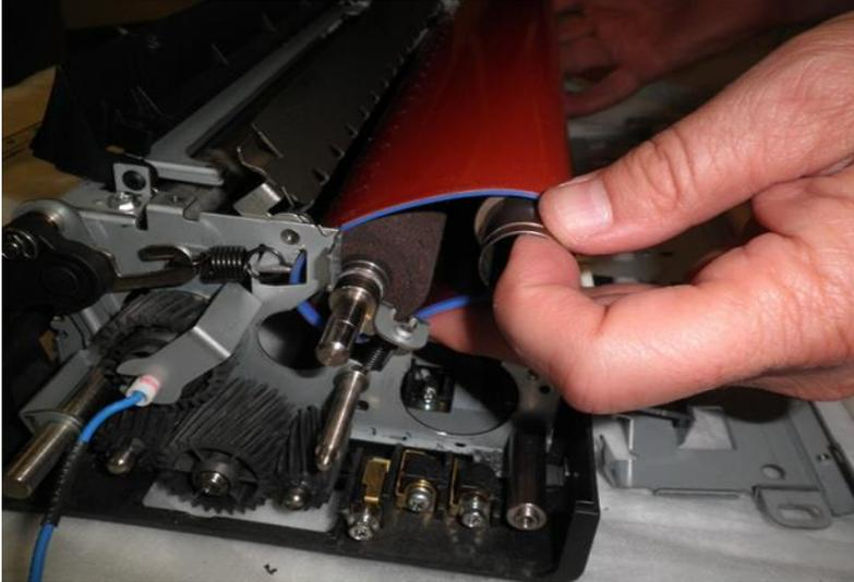
19. While applying tension to the belt, push the heat roller into its frame opening. Make sure both rollers are still in position between guide ribs:
