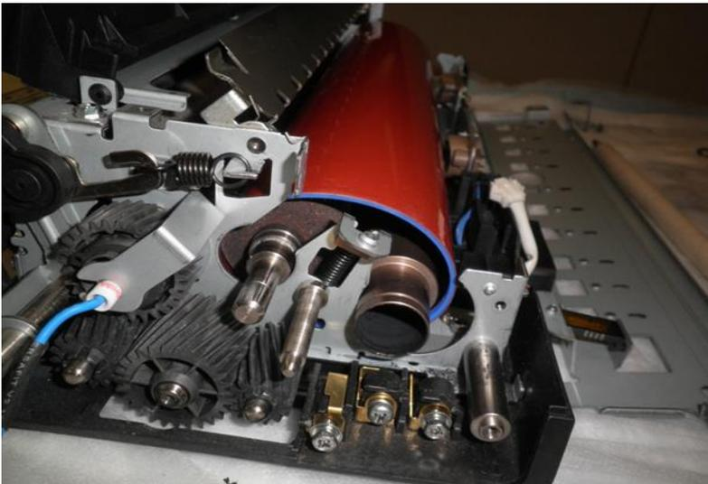
20. Slide the tensioner roller into the belt so that it is resting on top of the heat roller:
