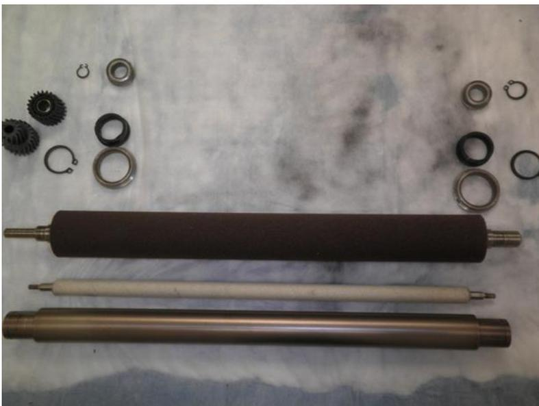
16. Place foam pressure roller and heat roller inside new belt:
