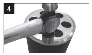
Position aluminum flange on new OPC drum and tap flange into position. Confirm flange is completely flush with drum substrate around the entire circumference. Repeat process to install second flange.
