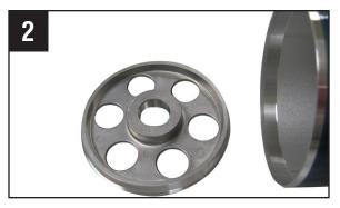
Remove aluminum flanges from used OPC drum by inserting a long screwdriver or small shaft/rod through one of the flange holes to tap out the flange on opposite end. Reposition used drum and repeat process to remove second flange.
