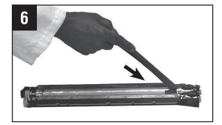
Remove all remaining residual developer from unit using a vacuum cleaner.
