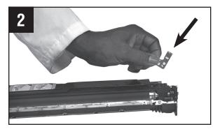
Remove ground plate after removing the screw securing it to the developer unit.
