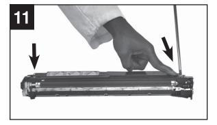
Re-position ground plate, making sure it makes proper contact with developer unit ground plate, then secure with previously removed screw.
