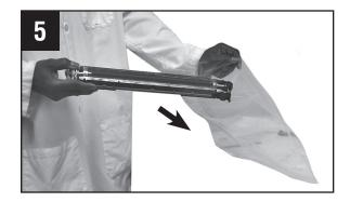
Pour used developer from developer unit into waste bag and dispose properly in accordance with local regulations (bag not included with Katun developer).
