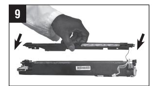
Replace cover plate by lining up tab grooves and snapping tabs into place.
