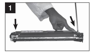
Disassemble developer unit by removing two screws from top of unit.
