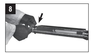
Rotate the developer roller to ensure even distribution of the developer on the surface of the developer roller.
