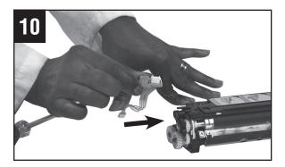
Reconnect white connector and reinstall connector bracket with screw.
