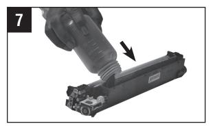
Pour new Katun developer into the developer unit, spreading the developer evenly across the length of the developer roller.
