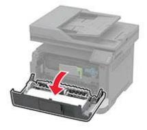
Remove the used imaging unit.
