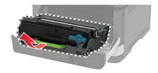
**3** Twist the blue latch, and then remove the toner cartridge from the used imaging unit.
