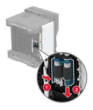
**9** Apply isopropyl alcohol to a soft, lint-free cloth, and then wipe the pick roller assembly.
