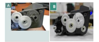
Depending on the cartridge you have, set gear as shown (SEE Figure A for the TNP-76,
