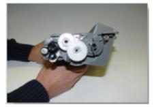
Re-install the developer roller with the long shaft to the gear side.
