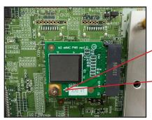
5. Insert the new eMMC (Katun PN 62161) and secure it with the original screw. IMPORTANT NOTE: Ensure the screw is tightened properly; an improperly secured screw may cause the machine to fail to recognize the eMMC.
