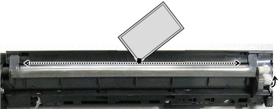
**7. Install developing unit in machine. Initialize and setup developing unit by following the instructions provided with Developing Unit Reset Chip (PN 39263).**
