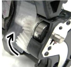
4. Position developing unit on a flat surface and vacuum remaining developer from developing roller surface.
