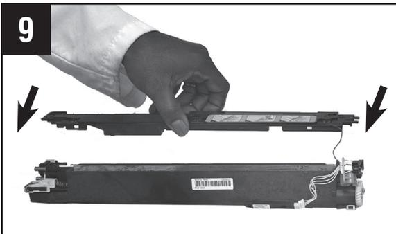
Replace cover plate by lining up tab grooves and snapping tabs into place.
