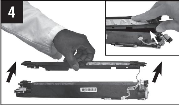
Remove cover plate by unsnapping clips along back of cover plate and lifting and loosening from ends.
