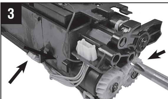
Remove connector bracket by removing screw; unplug flat white connector from the back of the lower unit.
