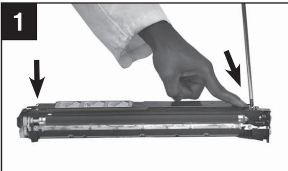
Disassemble developer unit by removing two screws from top of unit.
