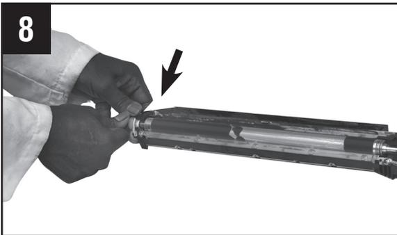
Rotate the developer roller to ensure even distribution of the developer on the surface of the developer roller.
