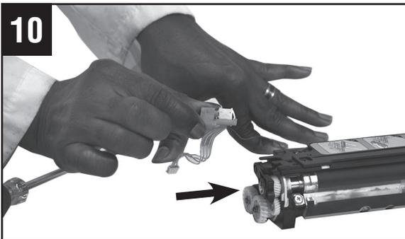
Reconnect white connector and reinstall connector bracket with screw.
