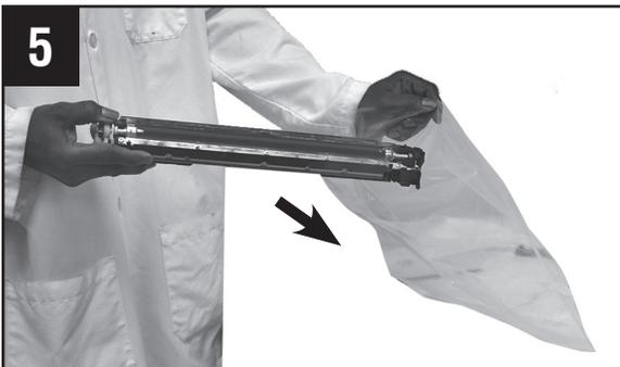
Pour used developer from developer unit into waste bag and dispose properly in accordance with local regulations (bag not included with Katun developer).
