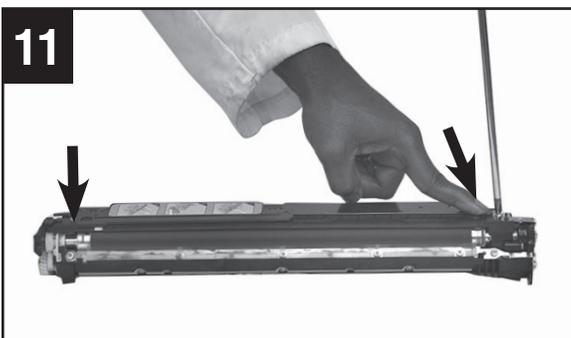
Re-position ground plate, making sure it makes proper contact with developer unit ground plate, then secure with previously removed screw.
